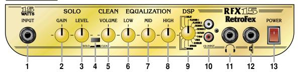
1: **INPUT**: Use this jack to connect your guitar to the amplifier by means of a shielded instrument cable.
